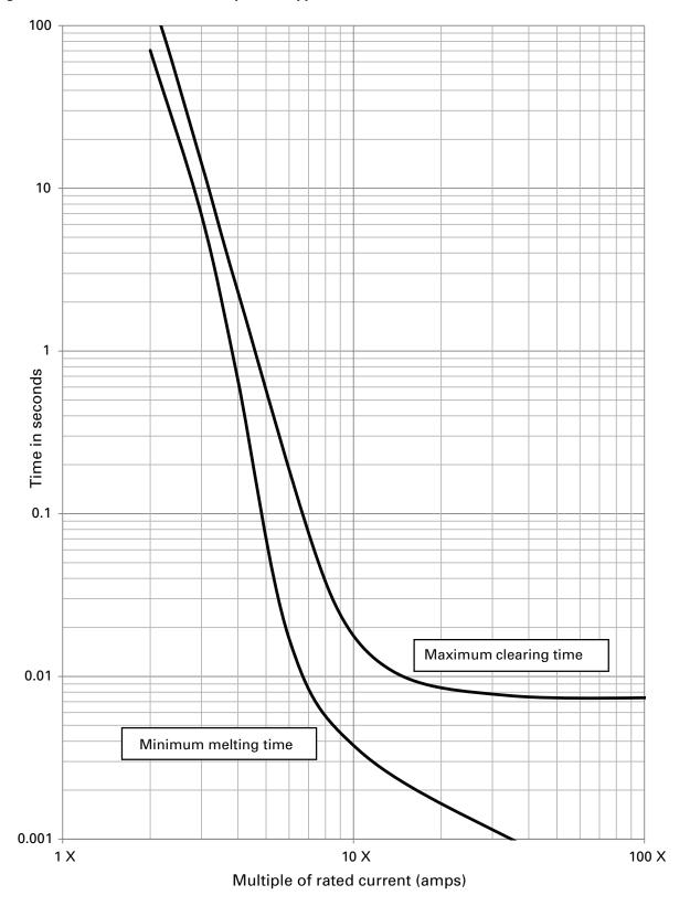
25 mm diameter DC minimum melt / maximum clearing time-current curves — multiple of rated current For catalog numbers EV25-100 to EV25-150 amp fuses supplied via DC rectifier @  $500 \, \text{Vdc}$  and time constant (L/R)  $2 \, \text{ms} \pm 0.5 \, \text{ms}$
