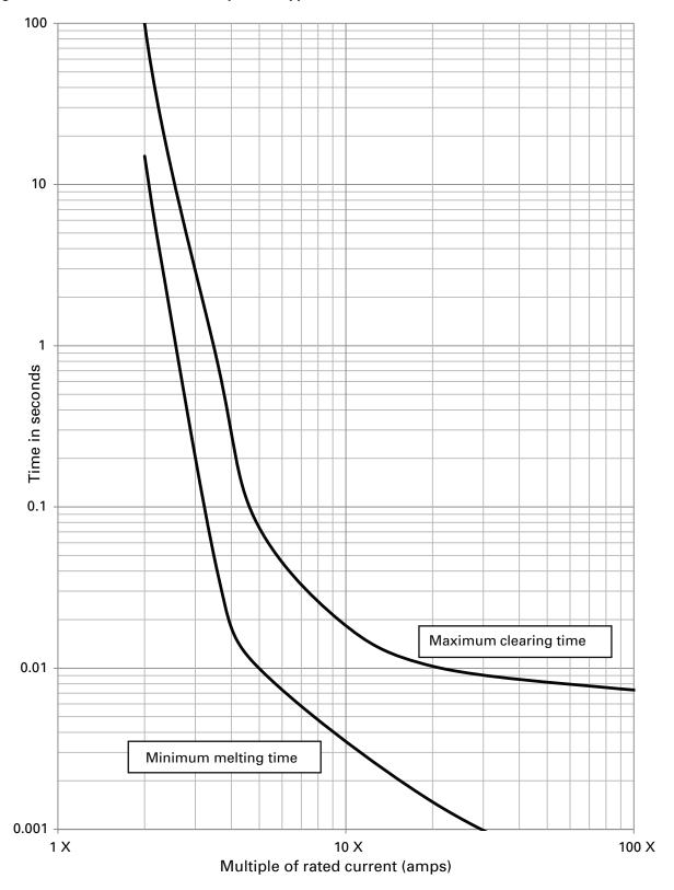
25 mm diameter DC minimum melt / maximum clearing time-current curves — multiple of rated current For catalog numbers EV25-175 to EV25-250 amp fuses supplied via DC rectifier @  $500 \, \text{Vdc}$  and time constant (L/R)  $2 \, \text{ms} \pm 0.5 \, \text{ms}$
