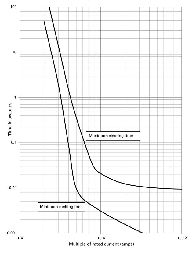
20 mm diameter DC minimum melt / maximum clearing time-current curves — multiple of rated current For catalog numbers EV20-125 to EV20-150 amp fuses supplied via DC rectifier @  $500 \, \text{Vdc}$  and time constant (L/R)  $2 \, \text{ms} \pm 0.5 \, \text{ms}$
