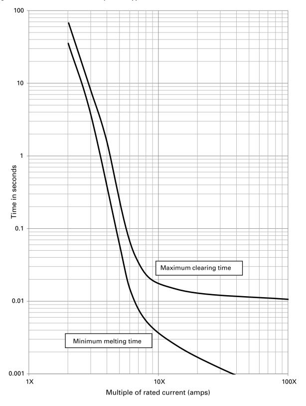
30 mm diameter DC minimum melt / maximum clearing time-current curves — multiple of rated current For catalog numbers EV30-200 to EV30-400 amp fuses supplied via DC rectifier @ 500 Vdc and time constant (L/R) 2 ms ± 0.5 ms
