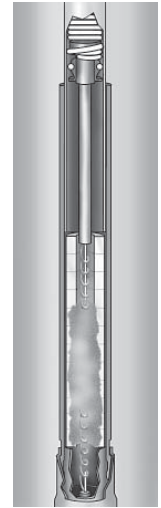
Vapor quenches arc at first current zero
